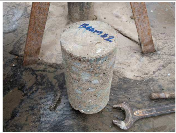
Fig. 6- Concrete sample extracted
