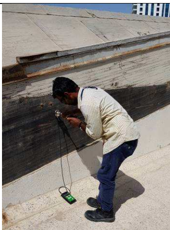
Fig. 7- Wooden Beam Testing
