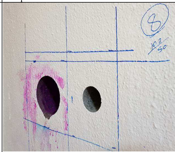
Fig. 4- Test Location 8 with Carbonation Depth
