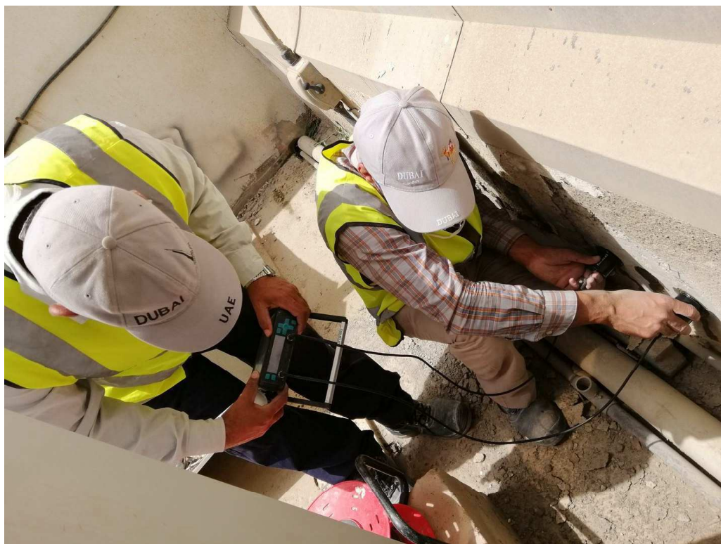
Figure 4-71 During measuring the Ultrasonic Pulse Velocity –Indirect
