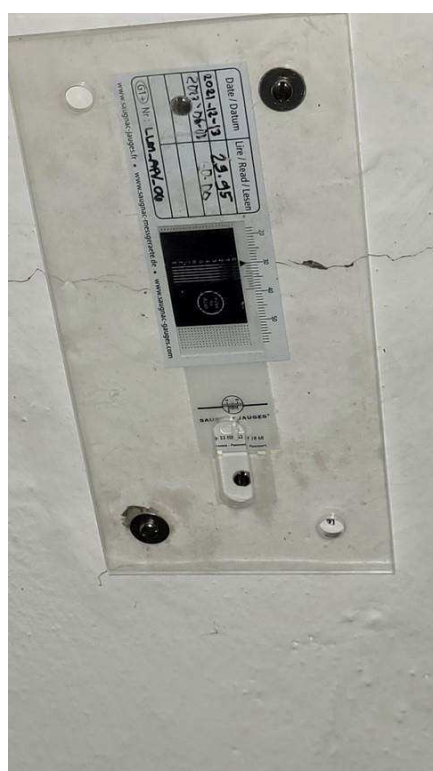
Figure 4-60 Cracks in concrete below stands
