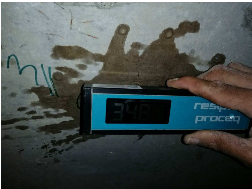
Figure 4-75 During measuring the resistivity
