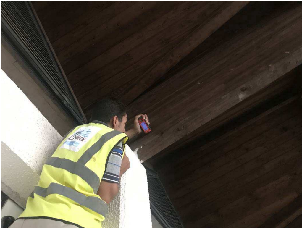
Figure 4-78 during checking the moisture content
