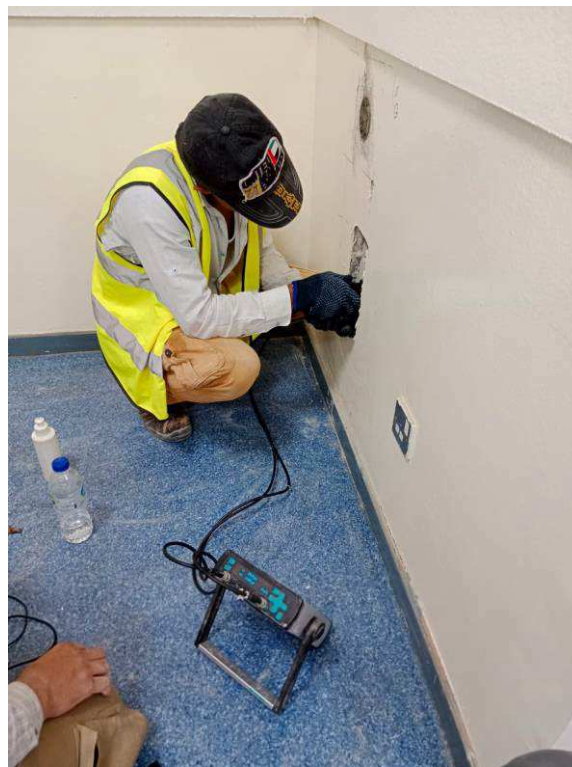
Figure 4-101 During measuring the Ultrasonic Pulse Velocity –Indirect
