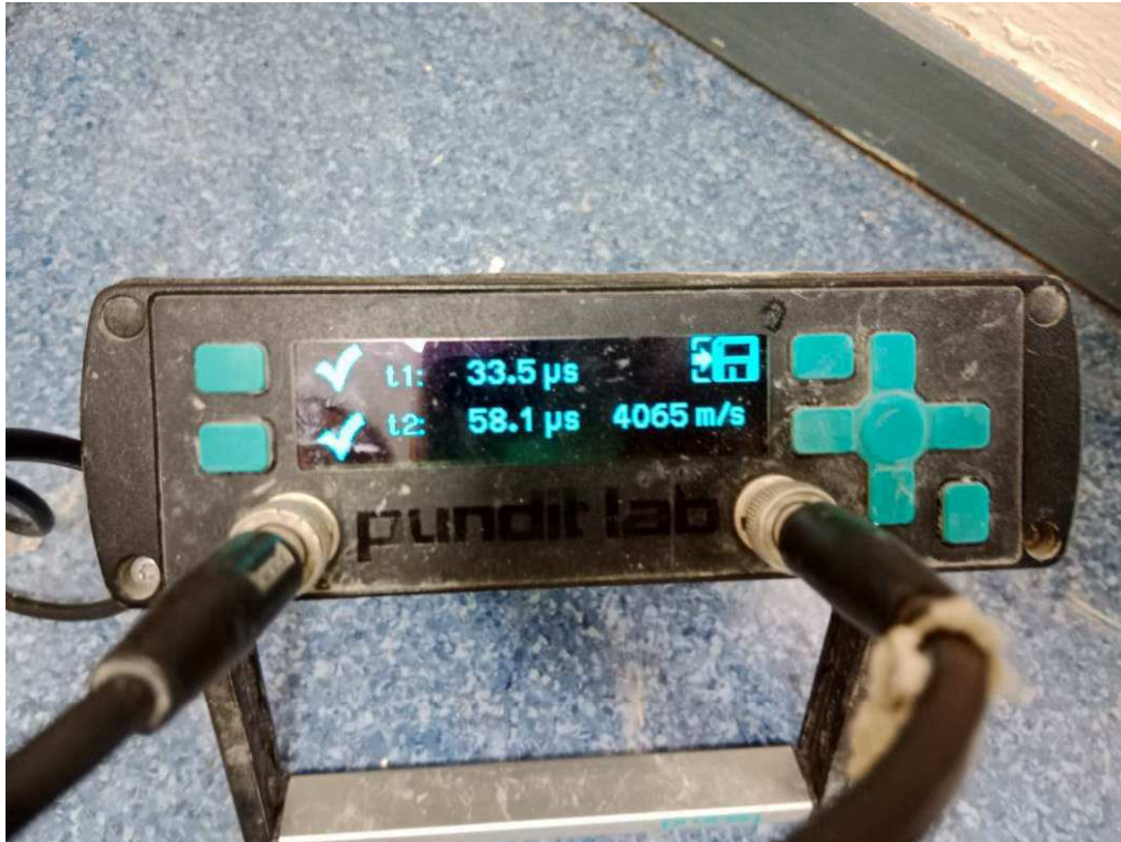
Figure 4-102 During measuring the Ultrasonic Pulse Velocity –Indirect
