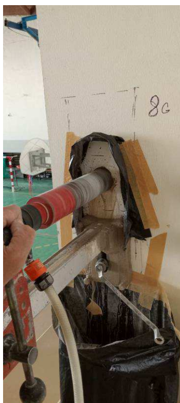
Figure 4-93 During coring the column
