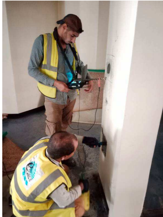
Figure 4-97 During conducting the half-cell potential test
