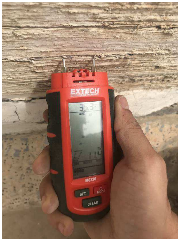
Figure 4-77 during checking the moisture content
