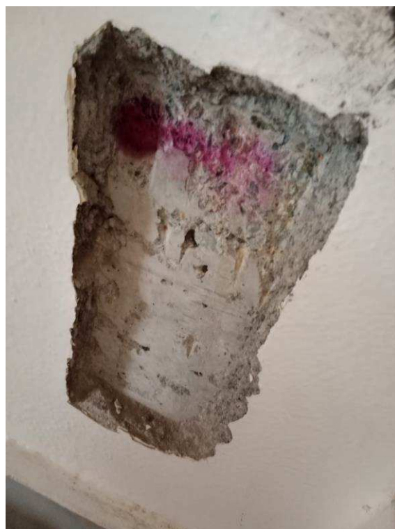
Figure 4-94 During the carbonation testing
