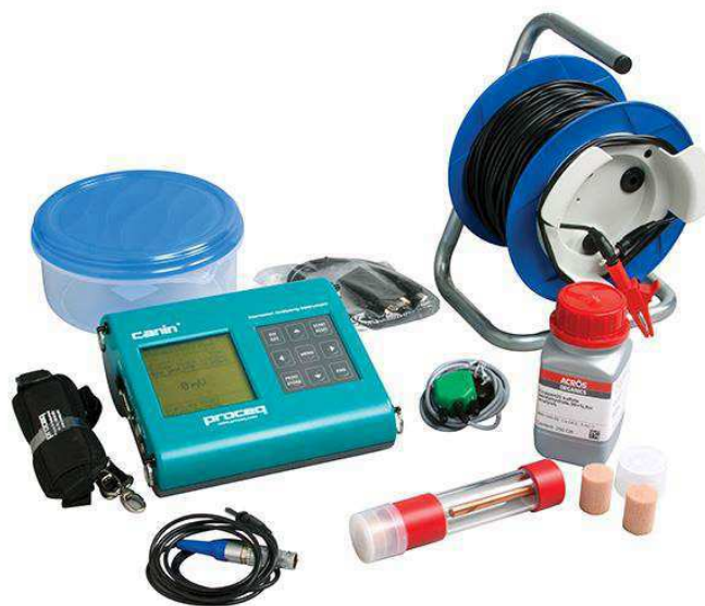
Figure 4-95 Canin system for measuring the potential
