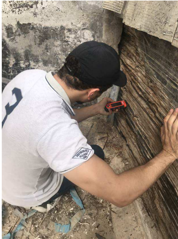
Figure 4-76 during checking the moisture content
