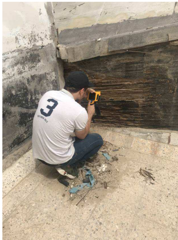
Figure 4-82 during conducting thermal image test over the damaged beam
